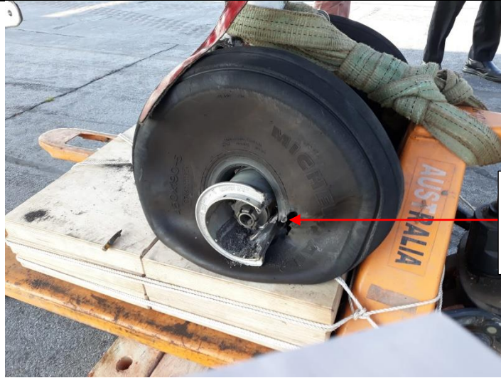
Nose Tyre - Ruptured and flattened
