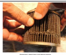
Photograph 5: Metal Chips in the filtering element
