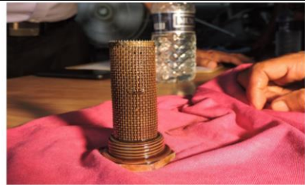
Photograph 2: Metal Chips on sump screen
