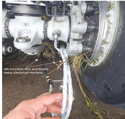
Figure 11 Electrical Harness pulled out
