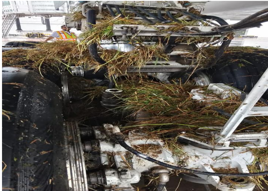
Figure-7 Left landing gear condition, forward to aft view after parking
