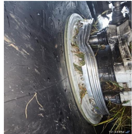
Figure 12 Damage to the Left-hand Brake Assemblies
