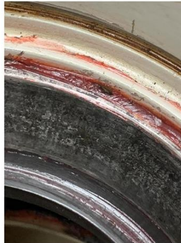
Heavy etching beneath smearing damage Figure 5
