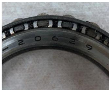
Roller ends in good condition Figure 2
