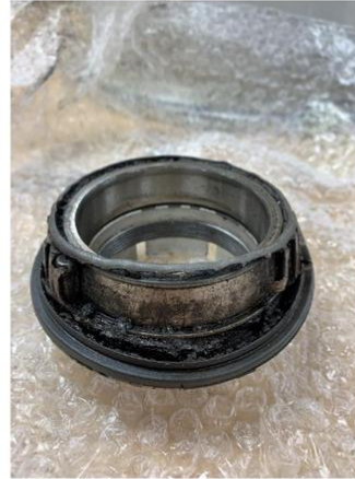
Cage bridges non-existent on half of cone Figure 5
