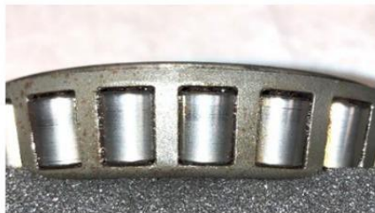
Very light frosting on roller bodies. Light corrosion on cage.
