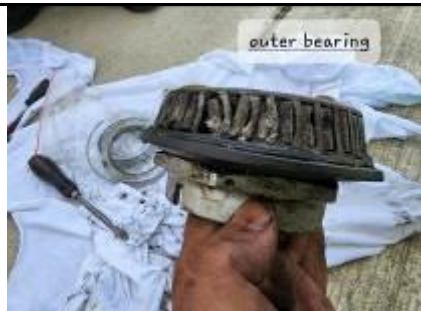
Figure-7: Damaged outer bearing.
