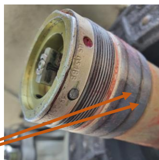
Figure-12: Scratch marks on the shinning portion of the axle throughout the shinning part circumferentially
