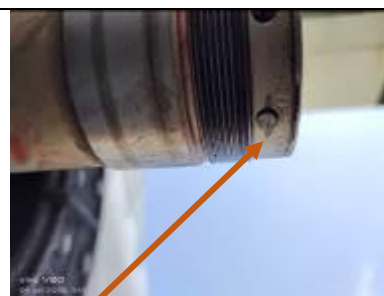
Figure-11: Lower part of the shearing locking bolt attached to wheel axle (Lower View)
