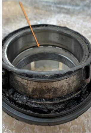
Cone and locknut welded together. Signs of corrosion and flaking paint near interface Figure 4
