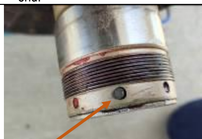
Figure-10: Lower part of the shearing locking bolt attached to wheel axle (Upper View)
