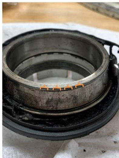
Roller spaced etching on cone raceway Figure 1
