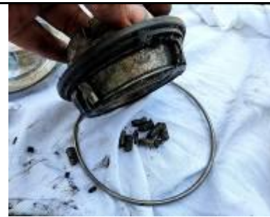
Figure-8: Damaged Roller.
