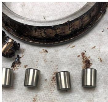
Grease is discolored, but appears to be in good condition Figure 1
