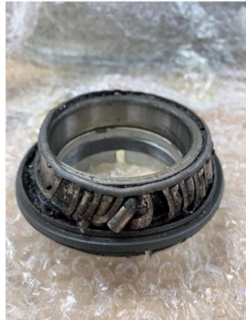
Cage and rollers skewed on half of cone. Fractured roller bodies Figure 6
