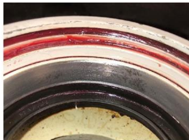
Light corrosion on cup raceway Figure 3
