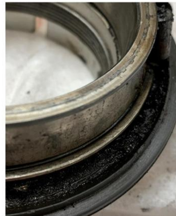
Corrosion on cone front face. Heavy scoring on roller ends Figure 7
