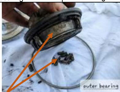
Figure-9: Traces of corrosion of roller and bearing.
