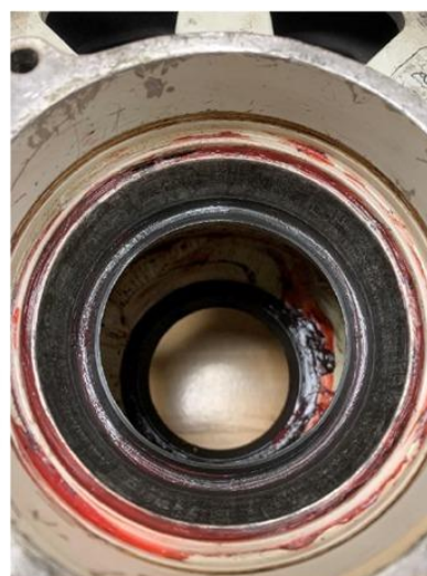
Etching and smearing around entire cup raceway Figure 4
