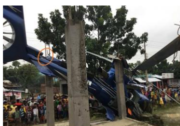
View from the back R/H side with the evidence of tail boom impact with a Main Rotor Blade
