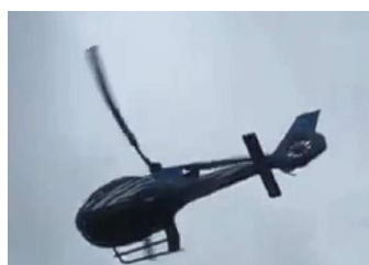
Aircraft just after take-off. Sudden right jerk and bank to the right observed (consistent with sudden loss of power).
