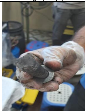
Photograph: (e) 03 (Shinning portion of broken bolt)
