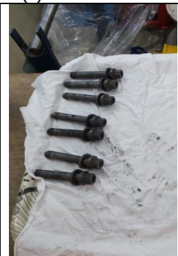
Photograph: (e) 05 (Seven broken bolts)
