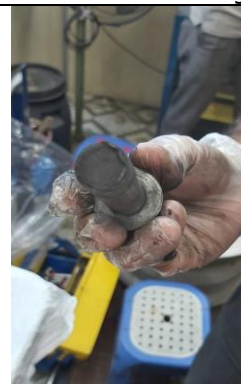
Photograph: (e) 04 (Full dullness of broken bolt)
