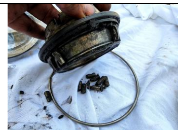
Figure-8: Damaged Roller.
