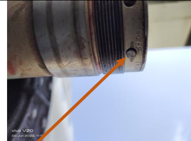
Figure-11: Lower part of the shearing locking bolt attached to wheel axle (Lower View)
