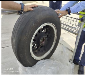
Figure-3: Inner side of the damaged wheel assembly.
