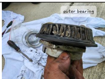
Figure-7: Damaged outer bearing.
