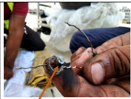
Figure -6: Upper part of the locking bolt with locking wire after removal from the wheel assembly.
